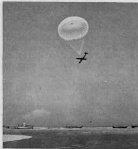
OQ-19D descending by parachute after control release.
